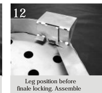
12 Leg position before finale locking. Assemble the remaining legs: pictures (1-4) and (8-12).
