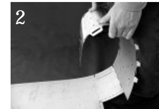
2 Bend and roll. Using thumbs and fingers. Shift your hands step-by-step (3-5 cm) forward.
