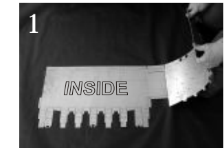
1 Turn the INSIDE up. Lift narrow end of the plate to knee height. Support the plate against your legs. Start bending and rolling.
