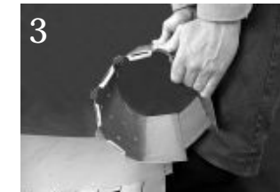
3 Shift your hands step-by-step (3-5cm) forward and complete the bending of the narrow part of the plate. If needed, repeat the bending (pictures 1-3)
